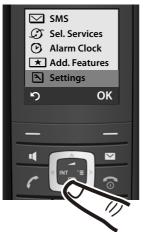
Press the bottom of the control key until Settings is highlighted by the bar.
