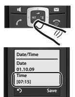
Press the bottom of the control key to scroll down to enter the time.
