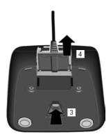
To disconnect the plug from the charging cradle, press the release button 3 and disconnect the plug 4.
